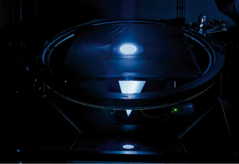
IBP photogoniometer for measuring the directionally resolved transmission and reflection properties of innovative facade components. © Fraunhofer IBP
