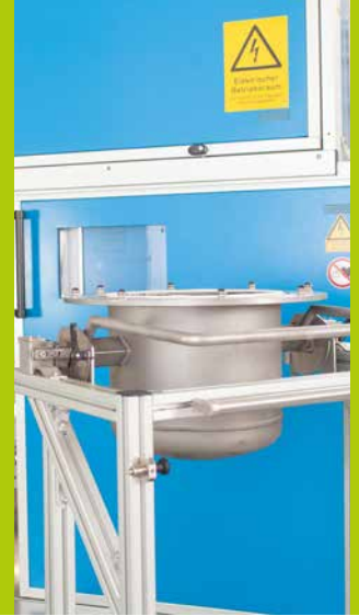
Electro hydraulic fragmentation device at Project Group IWKS: phase selective separation of recycling goods.
