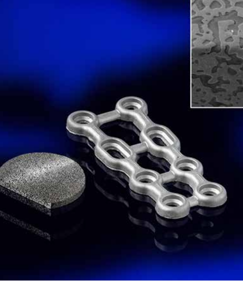
Porous disc and dense trauma implant made of biodegradable iron-TCP composite.
