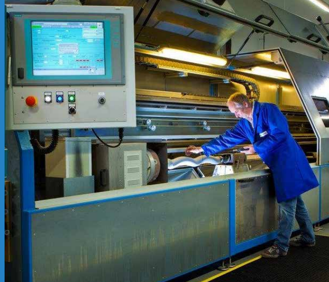
Finishing CFRP components by plasma spraying. © Fraunhofer IKTS
