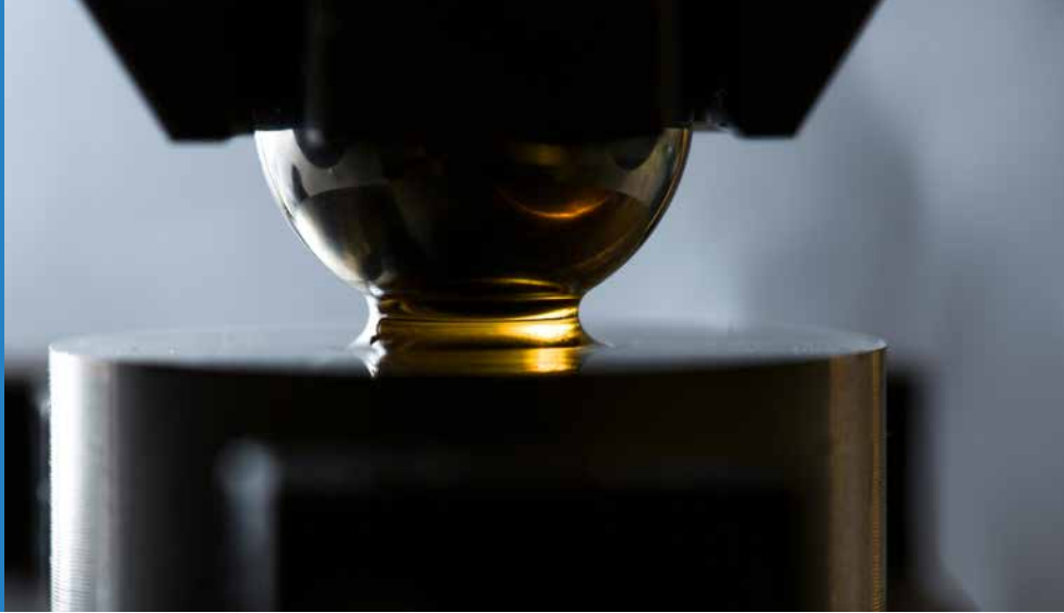
Ball-disc friction test in a vibration friction wear tribometer.
