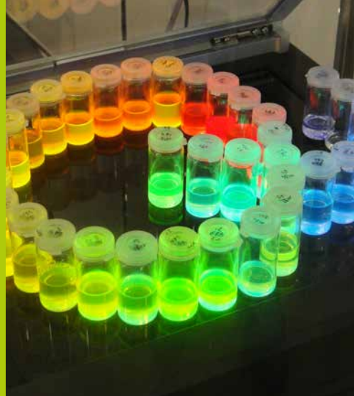
Quantum dots enable the manufacture of any color in a highly brilliant quality.
