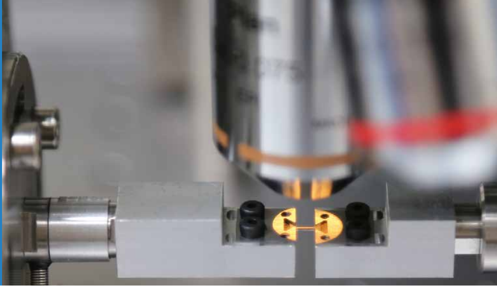
Micromechanical fatigue testing. © Fraunhofer IWM
