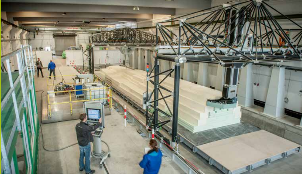
BladeMaker – integration, evaluation and demonstration of industrialized manufacturing processes for rotor blades.
