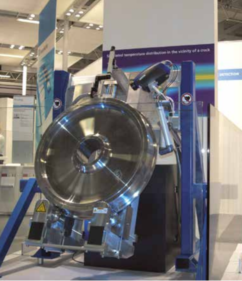
Demonstrator for active thermography on rail wheels.
