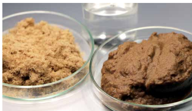
Starting material for wood foam: wood fibers and water are ground to a suspension and foamed.
