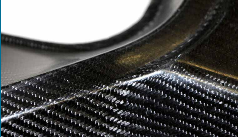
Carbon and hemp-fiber-reinforced composite. © Fraunhofer WKI
