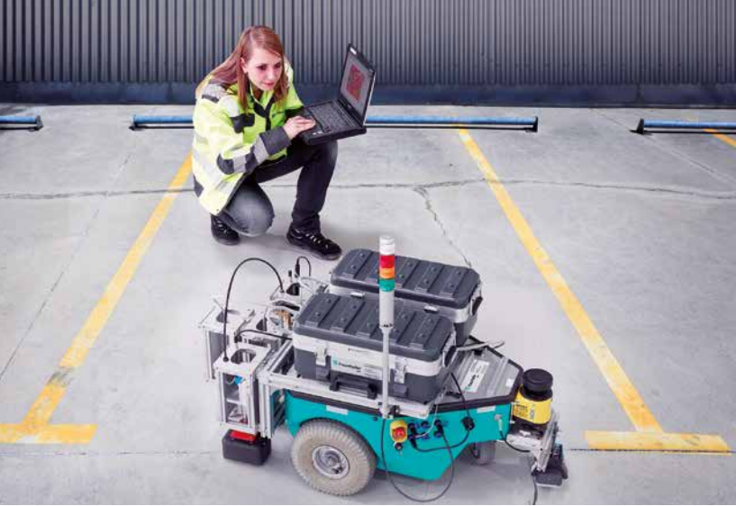
BetoScan – self-navigating robot for quick scans of large concrete surfaces. © Fraunhofer IZFP
