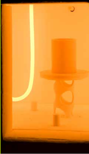
In-situ measurements of sintering processes in a thermo optical measuring system – survey photograph for the analysis of changes in dimension (right). © Fraunhofer ISC/Zentrum HTL
