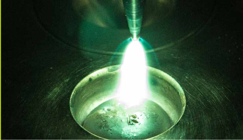
Manufacture of a new magnet alloy in an electric arc furnace. © Fraunhofer Project Group IWKS
