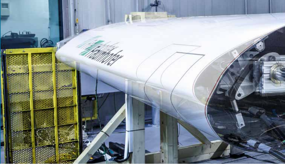
Droop nose demonstrator with a moveable wing leading edge and integrated future-oriented technologies.
