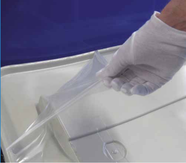
Removal of Flex PLAS ® release film from a fiber-reinforced component that has been coated in-mold with a gelcoat. © Fraunhofer IFAM
